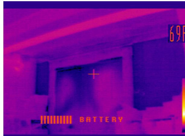
And then there's the connection to the attic. The ceiling has significant gaps in the air barrier – and there is an opportunity to increase effective insulation levels as well.
